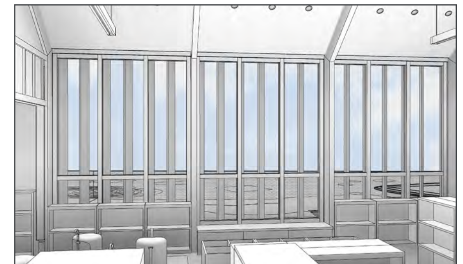
The barn with children's program space spilling out to the existing "play oasis". The large expanse of glazing with vertical shutters offers a visual connection between the interior and exterior, while providing necessary sun-shading and heat gain control.
