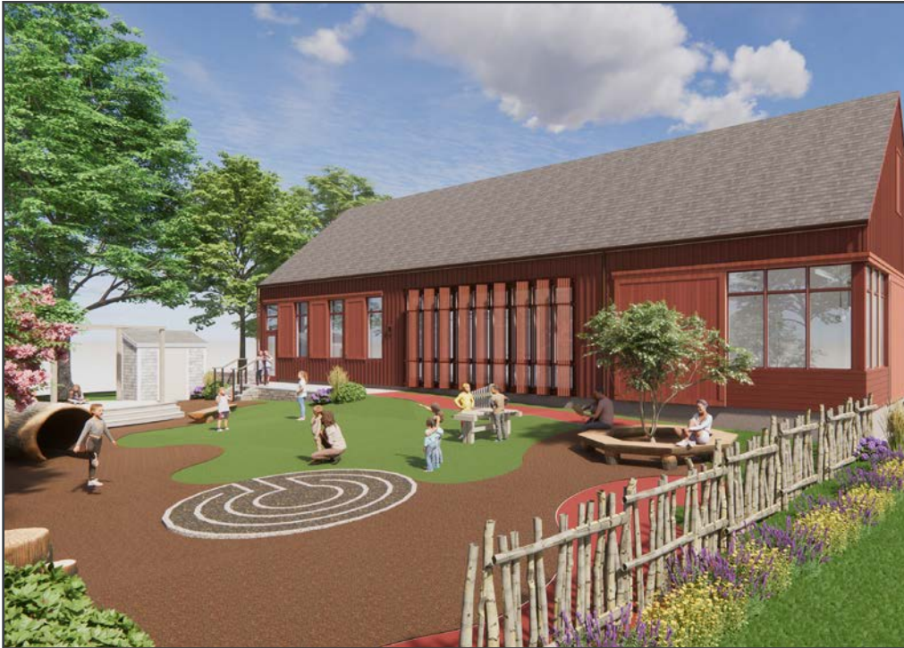
The barn with children's program space spilling out to the existing "play oasis". The large expanse of glazing with vertical shutters offers a visual connection between the interior and exterior, while providing necessary sun-shading and heat gain control.
